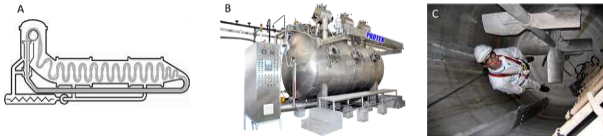
Figure 1. A. Schematic of a textile dyeing machine showing the route of the fabric through the equipment, B. Textile dyeing machine, C. Stirred tank reactor.
