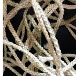
Figure 7. Suspected biofouling on lengths of polyamide 6.6 purse seine nets.
