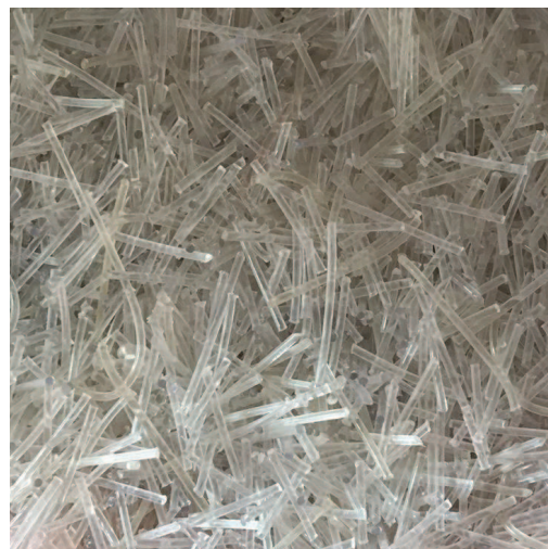
Figure 9. Hand-cut (shredded) polyamide monofilament gillnets.
