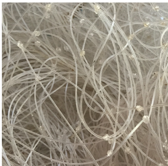
Figure 8. Polyamide monofilament gillnets sourced from MCB Seafoods.
